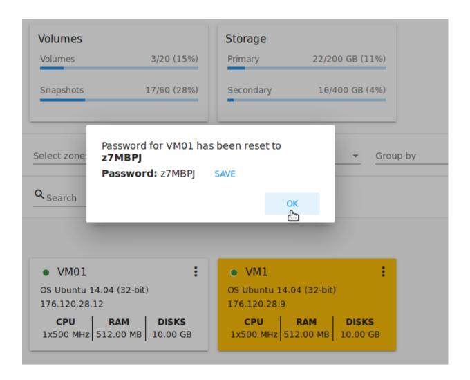
• Access VM - Opens an "Access VM" dialog window which allows to view VM name and IP, view and save a password for the VM and access the VM via the VNC console.
